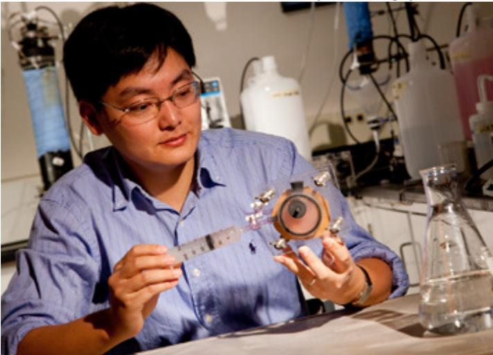
Zhen He, UWM assistant professor of engineering, is developing a microbial fuel cell that generates energy while simultaneously purifying industrial wastewater. He's research is one of the projects suggested to industries in the new I/UCRC.
